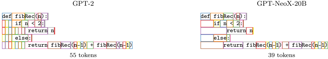
Figure 3: GPT-2 tokenization vs. GPT-NeoX-20B tokenization. GPT-NeoX-20B tokenization handles whitespace better, which can be particularly useful for text such as source code. For more examples, see Appendix C.
